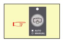
② By pressing "AUTO button" of CTTS-801 Controller, Proceed as Auto mode. Under Auto mode, Green Lamp is on.
