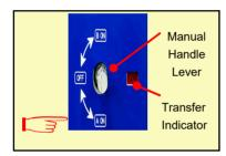
③ Transfer the switch by using and turning Manual handle lever to A-ON(Counterclockwise)
